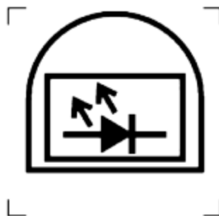
Figure 1 – Symbol for built-in LED modules
